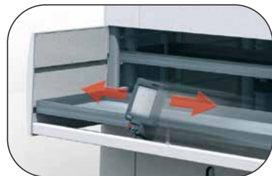
2 Optional sliding console: functional and ergonomic to help the operator during intensive picking activities
