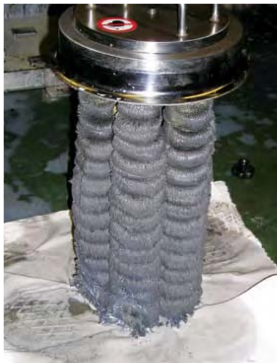
A magnetic filter element showing fines collected from fluid, after conventional filtration. (Photo courtesy of Knoll America)
